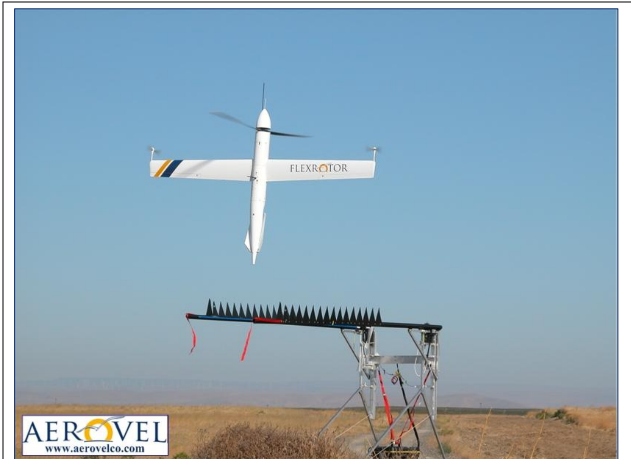
Pandora , Aerovel's Flexrotor prototype, hovers over her handling rig. The rig assembles in a few minutes out of a duffel bag, and is designed to complement Flexrotor 's airborne autonomy with fully automatic retrieval, fueling, checkout, and launch.
